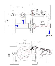
**NOTE:** To allow for maintenance while installed, the Model C-EL shall have a free space of 2/3rds its length (L2) at the valve trim side.
