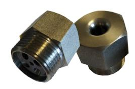
All internal water ways have diameters larger than 3mm. Nozzles should only be utilized in pipe systems with clean internal pipe surfaces and cavities. Nozzles should be installed in systems with a main-line water strainer with mesh size equal to or less than 3mm.
