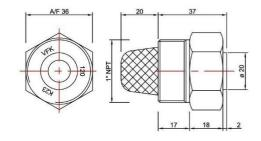
Only Naval Brass and Titanium nozzle w/stainless steel or titanium strainer are FM Approved
