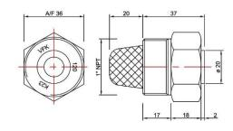
Only Naval Brass and Titanium nozzle w/stainless steel or titanium strainer are FM Approved
