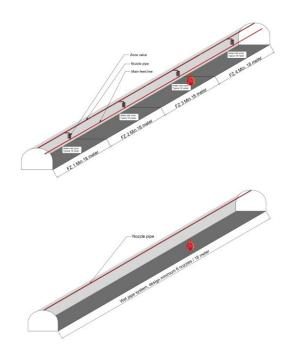
Water consumption using Nozzle CT-ODC1, open pendent nozzle shall be designed based on minimum 2 zones of 18 meter or more. It is however recommended to design with 3 zones.
