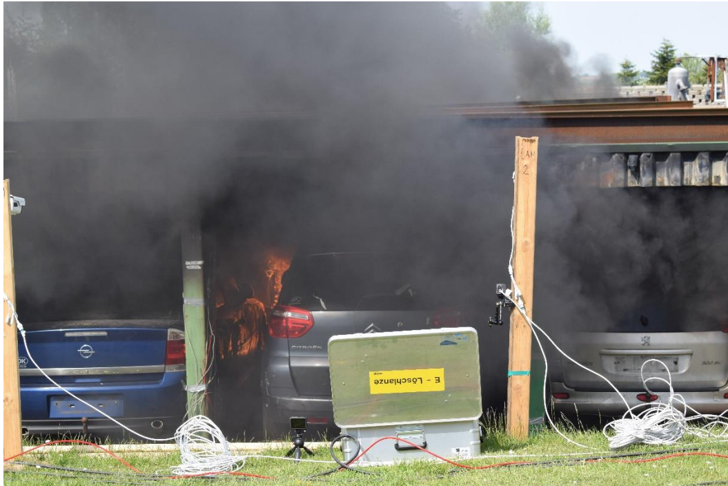
Fig. 2.2 Tesla fire developing.
