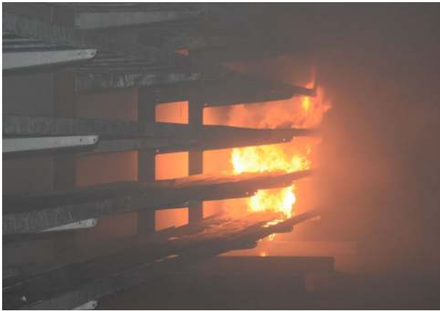
Fig. 2 Cable tunnel fire test
