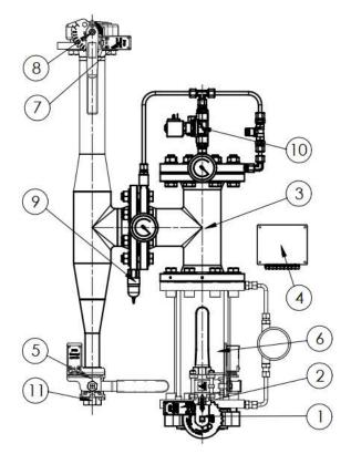
The Model Tunprotec C-M-80-50-S features small outer dimensions, robust and reliable components, and the ability to remotely activate the zone control valve and allowing the fire zone control valve to be monitored remotely through relay switches.
