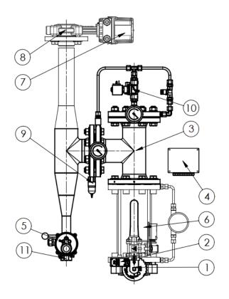
The Model Tunprotec C-M-80-50-I features small outer dimensions, robust and reliable components, and the ability to remotely activate the zone control valve and allowing the fire zone control valve to be monitored remotely through relay switches.
