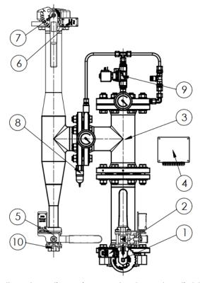
The Model Tunprotec C-M-80-50-I-NF features small outer dimensions, robust and reliable components, and the ability to remotely activate the zone control valve and allowing the fire zone control valve to be monitored remotely through relay switches.
