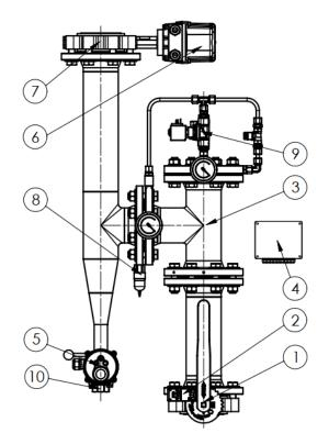
The Model Tunprotec C-A-80-80-I-NF features small outer dimensions, robust and reliable components, and the ability to remotely activate the zone control valve and to have it run a self-test sequence in which activation and alarm functions can be tested.
