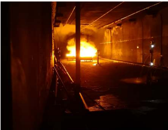
Full scale tunnel fire testing at APPLUS test center in san Pedro de Anes in Spain
