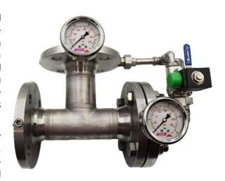
The Control Valves have been designed with the intention of being installed in fine water spray fixed firefighting systems (FFFS) in commercial and industrial applications. Because of the stainless-steel housing and internal components, the Model C-EL Control Valves are highly applicable in most areas. The valve can easily be disassembled for easy maintenance and refurbishment, without removing the valve housing from the connected system.
