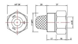
Only Naval Brass and Titanium nozzle w/stainless steel strainer are FM Approved
